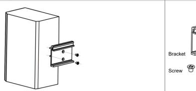
Step b: Install the device to the DIN rail.
