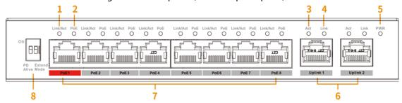
Following are all the ports and indicators on the front panel of the 4&8-port unmanaged desktop switch (without optical ports), and might differ from the actual product.
