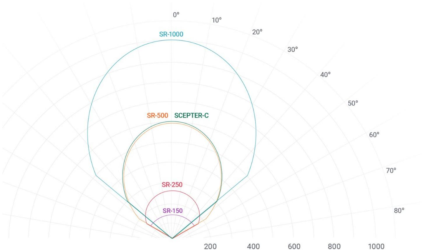
Figure 6: SR-Series Maximum Coverage Diagram (Top View)
