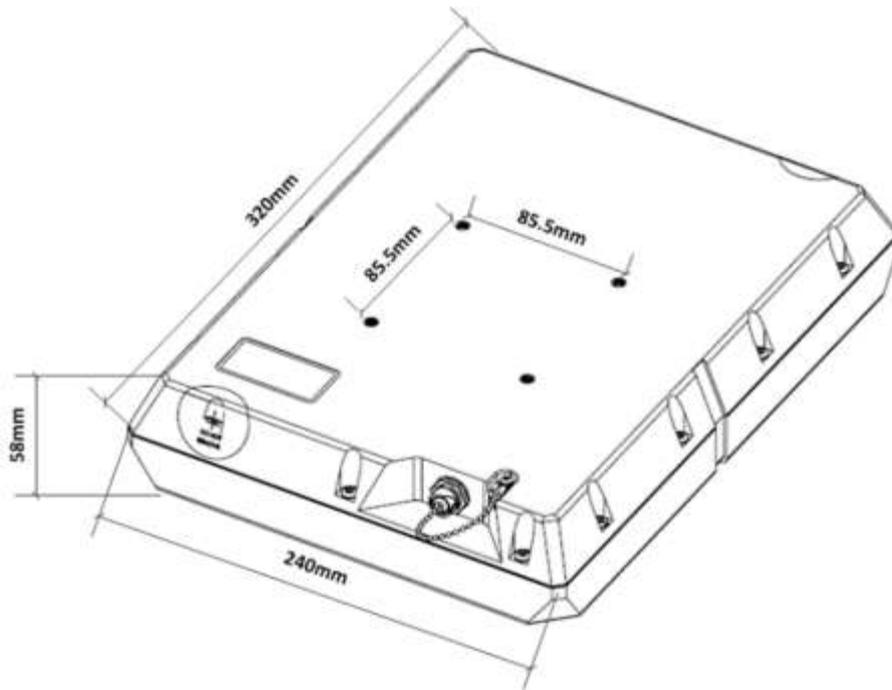
Figure 3: SR-1000F/SCEPTER Mechanical Dimensions and Mounting Holes
