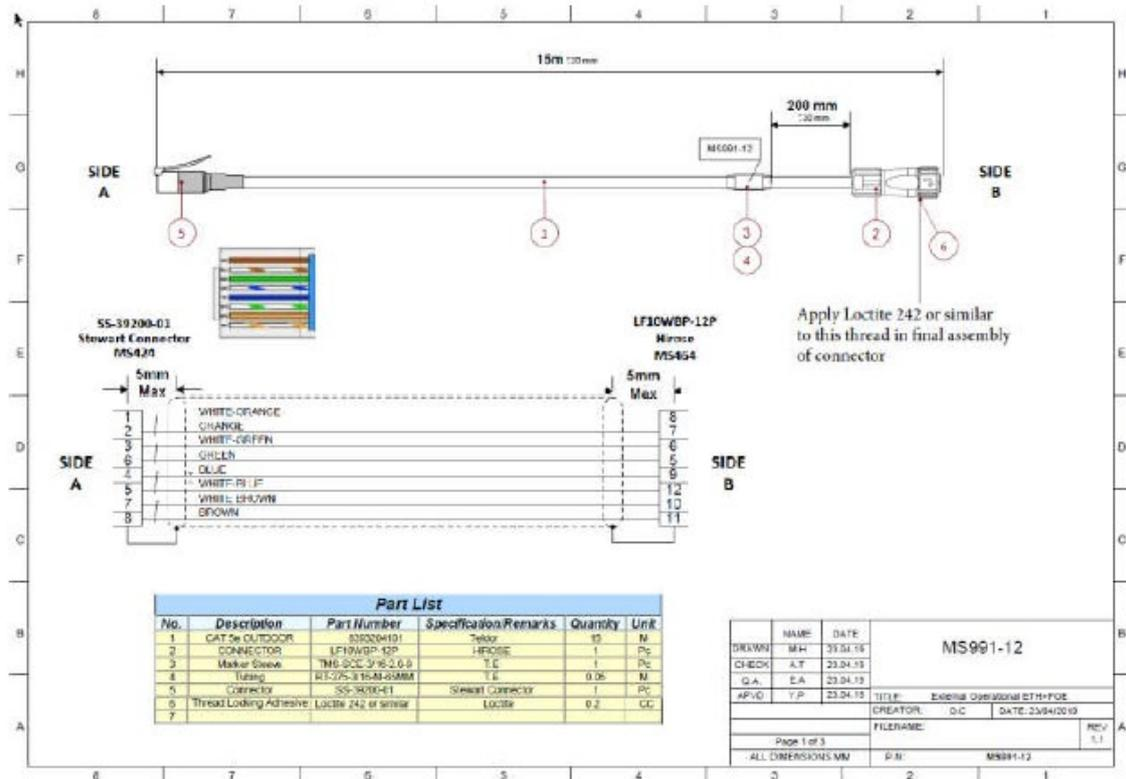
Figure 8: SE-Series External operation cable
