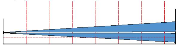
Using the sensor with 2 vertical curtain lenses: the use of vertical curtain lenses is based on the need to protect doors and windows with a vertical curtain that is no wider than 50 cm. In this way the protection is only near the doors and/or windows without extending into other areas. You can position the sensor at a height of between 1 m and 2 m based on need. The beam is about 50 cm wide for an aperture of about 90/100 vertical degrees (fig. below)
