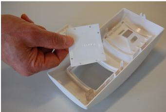
Position the new lens in the housing, replace the funnel and snap it into its housing.
