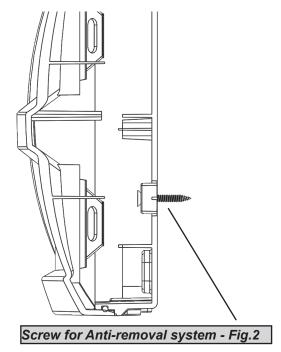
Once the cable and wall attachment holes have been made, take the measurement to attach an anchor (3 mm) to the anti-removal system. (see above fig. 1 and fig. 2)
