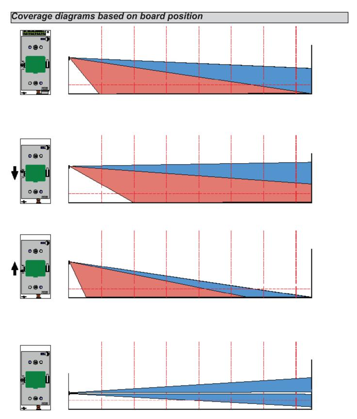
Note: the figures show the effect of the beams based on the position of the board. Since they are purely indicative, we recommend you thoroughly test the sensitivity of the sensor after each adjustment.
