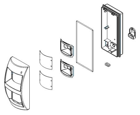
To replace the lenses you must remove the funnel and remove the lens that is resting in the housing as shown in figure 1 and 2.
